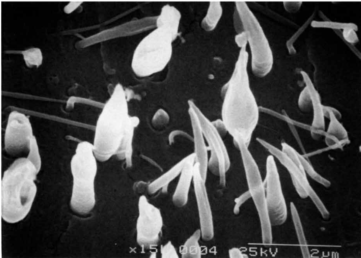
Figure 9 (a) SEM picture of PC/LC10C blend. Spinning temperature of 260°C; draw ratio of 20; magnification of 5000×. (b) SEM picture of PC/LC10C blend. Spinning temperature of 260°C; draw ratio of 20. A view at magnification of 15,000×.
